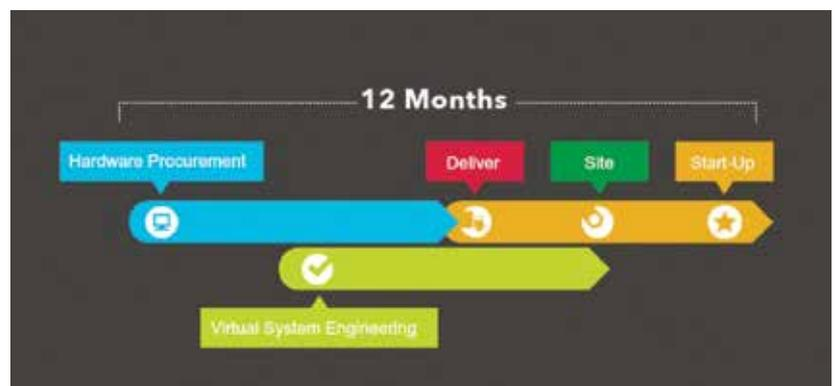
Enabling hardware procurement and system engineering to proceed simultaneously can reduce typical project implementation times from 18 to 12 months.
